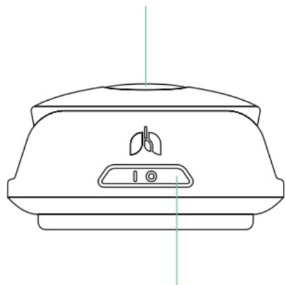
2. Control button - turns it on/off, connects to the app, starts a recording
