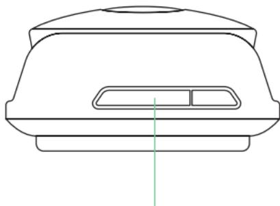
3. Micro-USB port (covered by a protective flap) - used for charging
